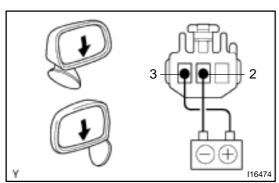
(d) Reverse the polarity, and check that the mirror turns upward.
