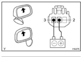
(c) Connect the positive (+) lead from the battery to terminal 2 and the negative (-) lead to terminal 3, and check that the mirror turns downward.
